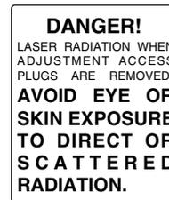
Non-interlocked Protective Housing Label for Adjustment Access Plugs (4)
